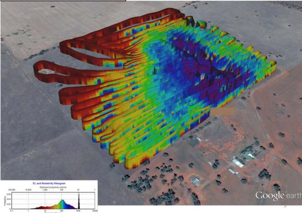
Figure 7 An example of hard rock (Monzodiorite) definition using mine-scale TEM survey (20m spaced lines).
