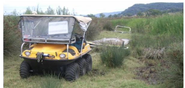
Figure 2 A Slingram TEM system designed for rougher terrain, easy setup and packup, and with ability to be driven through narrow gaps.
