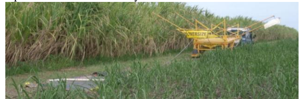
Figure 1 The AgTEM2 (Groundwater Imaging 2010) survey platform during early trials. The platform is designed to quickly transform from road legal form to survey capable form. It is designed to resolve a large depth of investigation from 1m to 100m (and in the future potentially 100's of metres). Booms fold in and out via remote control. The Trailer, made of fibreglass, has a drawbar which extends to separate the closest transmitter loop edge from the towing vehicle by 5m raising its ground clearance to over 1m as it does so.
