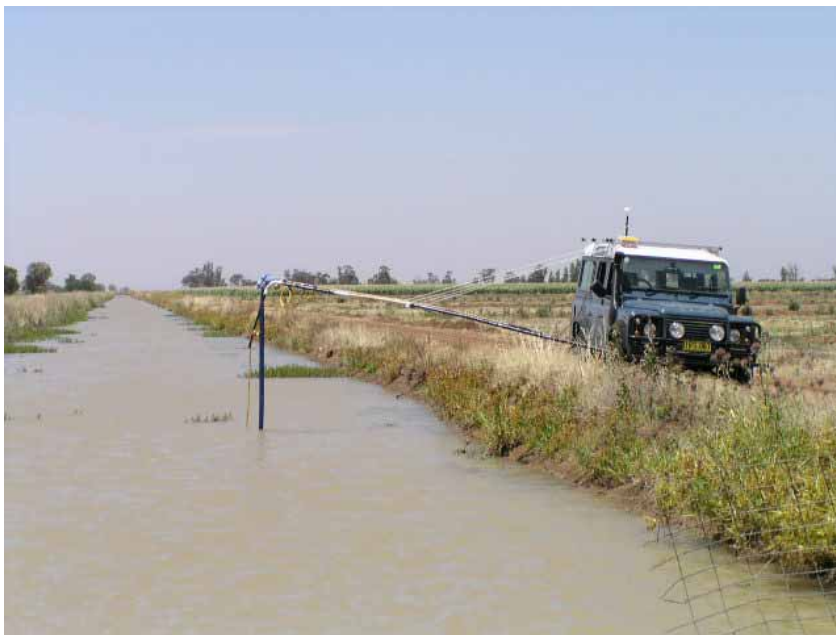
Figure A2-3 The boom towing an array along a weed filled irrigation canal.
