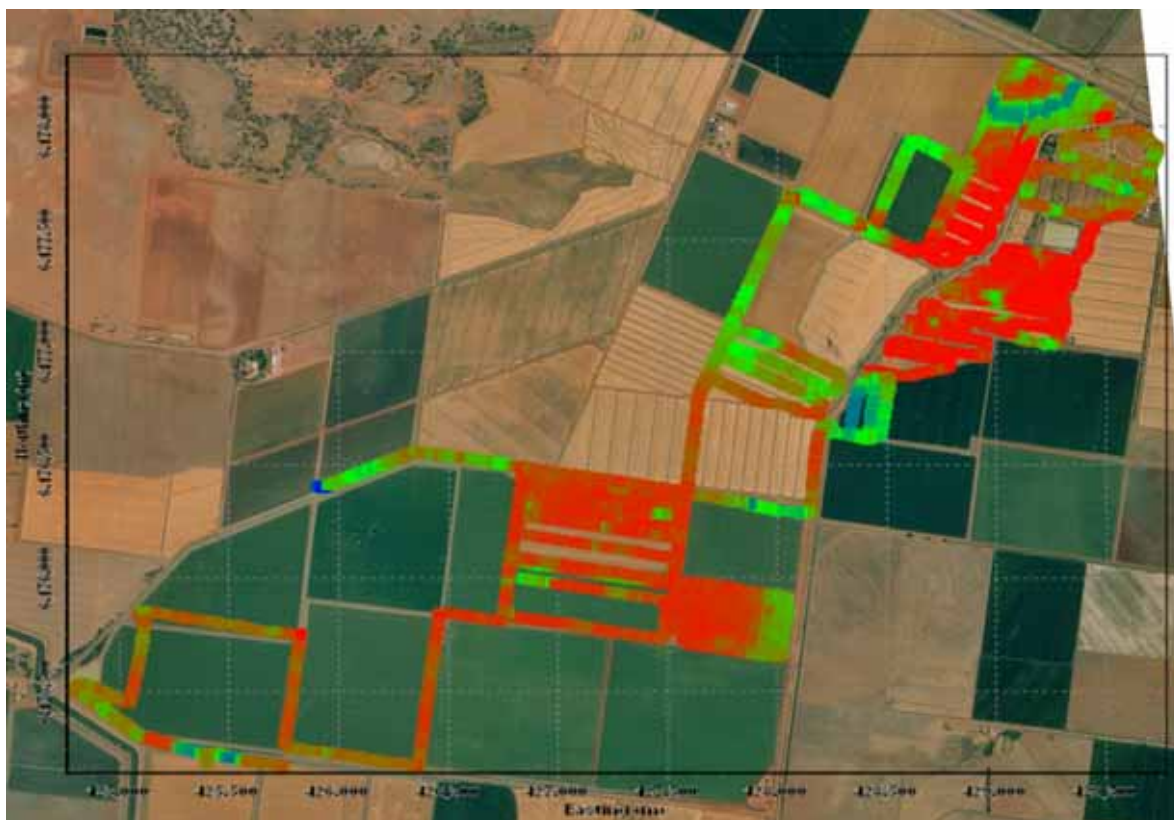
Figure A9.2 Towed NanoTEM EC slice at a depth of 8 metres – Dallas Clay Pan. Red represents high EC, Blue represents low. Note strong correlation with the floating AXB array data presented in Figure 17-7 of the Chapter 17 ‘Networks of farm canals and drains’.
