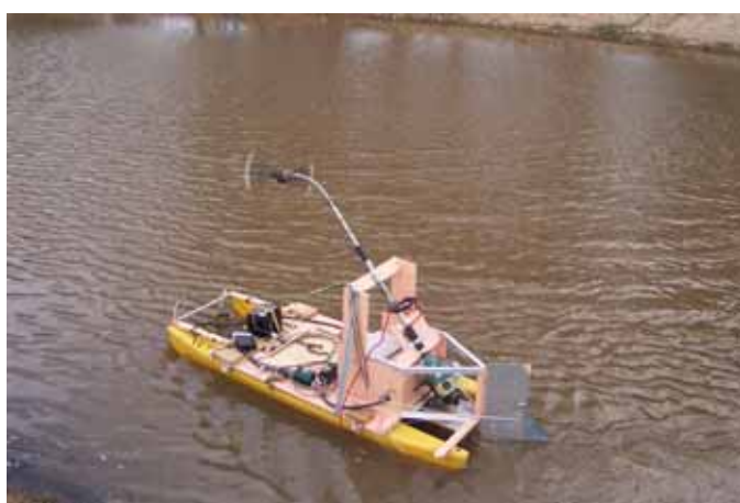
Figure A2-15 A close-up of a experimentation leading towards a radio controlled platform designed for geo-electric surveying.
