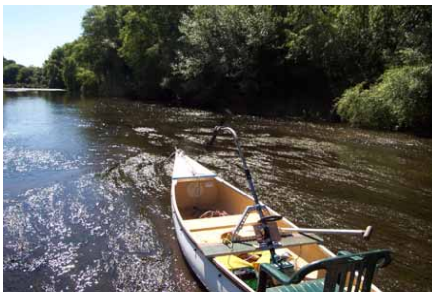
Figure A2-8 A prototype small scale air-propeller propelled canoe capable of negotiating weeds without fouling shown here crossing rapid filled shallow rapids in the Macquarie River. This prototype is being scaled up and refined to produce a useful survey device.
