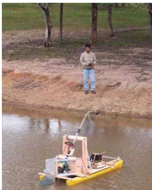
Figure A2-14 Experimentation leading towards production of a radio controlled platform for geo-electric surveying in weed filled canals. Note the 18” propeller attached to the grass trimmer used for initial experimentation.
