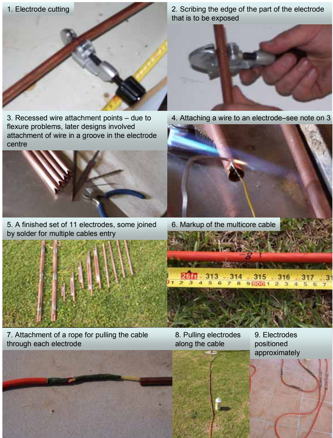
Figure A1-1 Towed geo-electric array construction – part 1.
