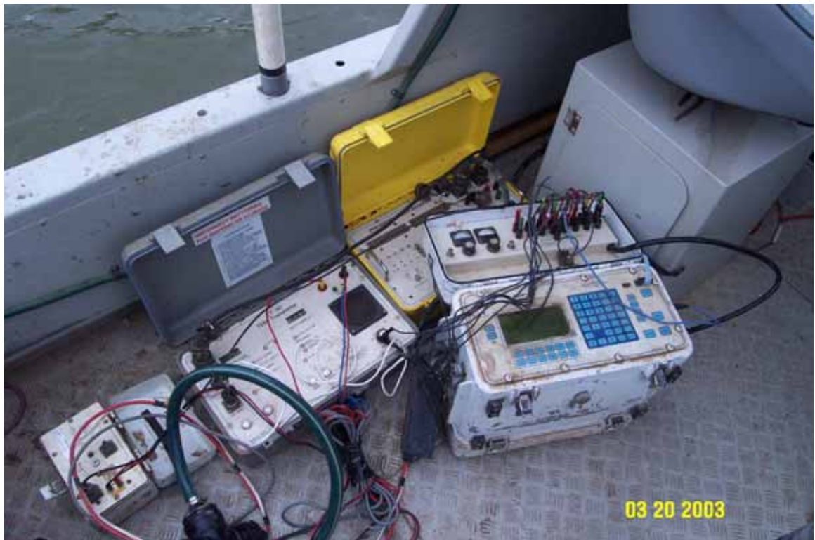
Figure 7.7 Zonge GDP32 Receiver, isolation amplifier, shunt resistor, signal generator and voltage booster.
