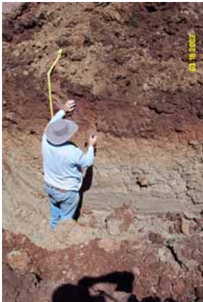
Figure 17.11 Mike Nalore examining soil investigation trench site 7. Note the base of the red soil where some gypsum exists. Once this trench was extended past 5m deep, so much water was gushing in that it had to be abandoned. Permeability exists there in clay structure. The clay had aggregated into grains between which water could flow.
