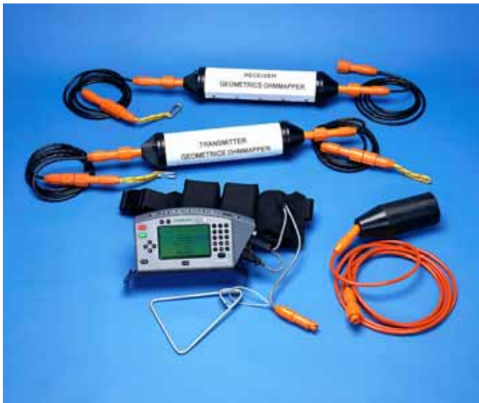
Figure 8.3 The Geometrics Ohm-mapper capacitive coupled resistivity imaging equipment. Only one receiver dipole is shown. The linear electrodes are actually the cables, not the pods.
