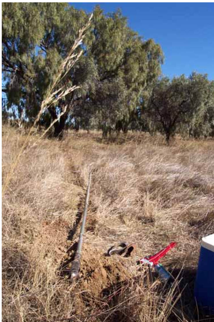
Figure A7-3 A three metre auger sampler, and bits for various soil types. (Bundure canal inferred seepage site).
