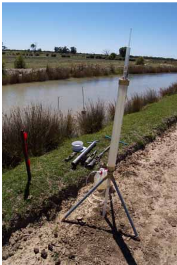
Figure A7-11 A Guelph Permeameter with an Idaho seepage meter in operation in the background.
