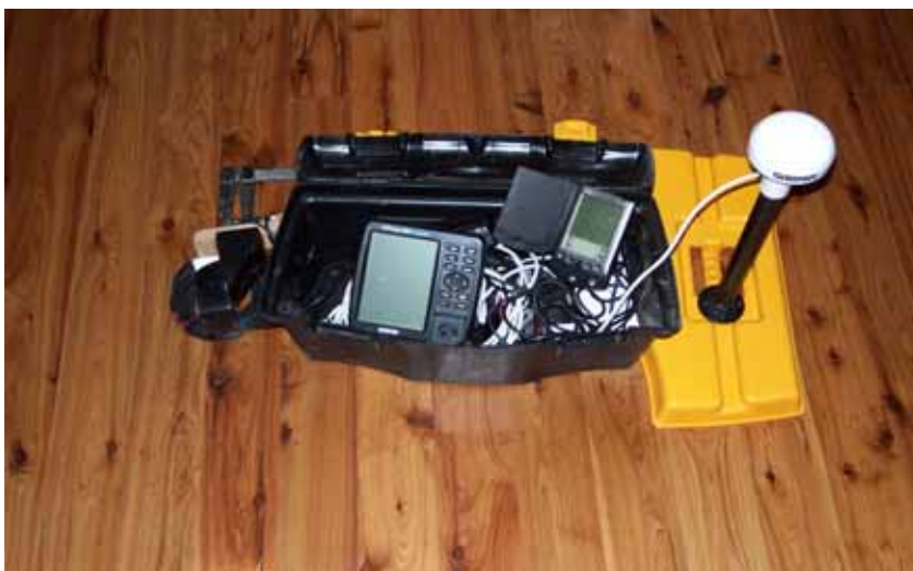
Figure 7.5 The GPS and sonar (Garmin GPSMap188) and data logger (PalmVx) subsystem
