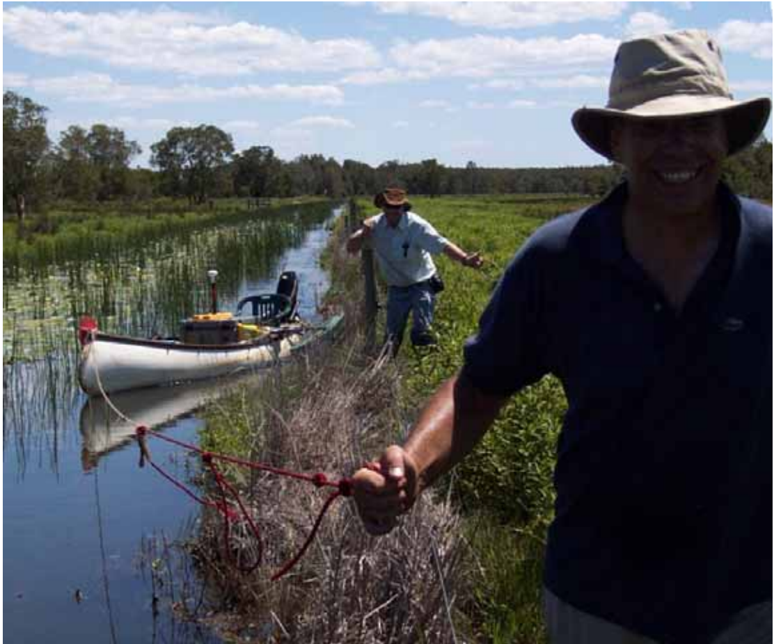
Figure A2-10 Pulling a canoe along an acid sulfate and acid loving weed filled swamp drain in a skewed manner using an outrigger and ropes to keep it away from a canal bank while straddling an electric fence. The canoe is towing a functioning 144m array. The outboard motor would not function in this weed. This looks hard but is actually fairly easy and fast. It is easy to see how an alternate motorized propulsion device could improve productivity in situations like this.
