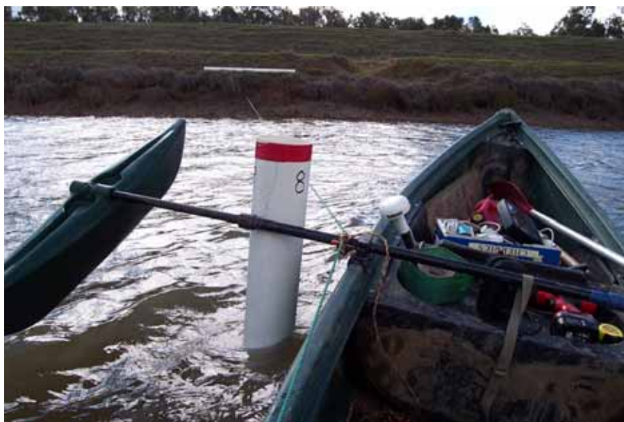
Figure A7-8 Installation of a vertical pipe infiltrometer or SPOT.
