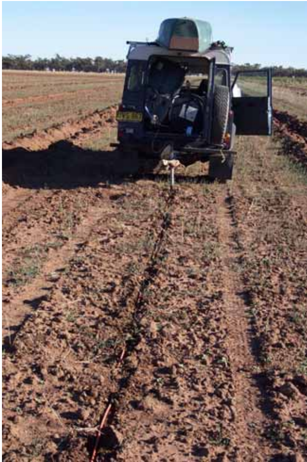
Figure 8.6 Towing of a geo-electric array using a ripping tine. Slightly deeper ripping and addition of a press wheel is needed to prevent the array from leaving the ground as it does here.
