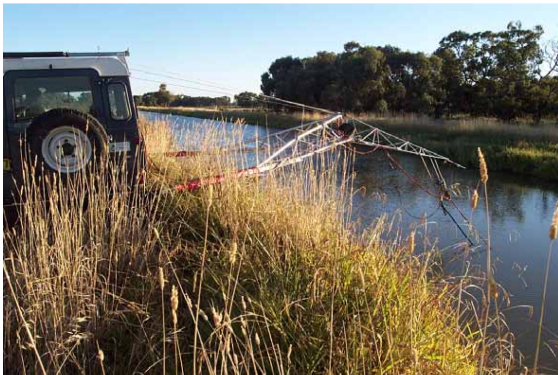
Figure A2-7 A recent enhanced boom design with a 6 metre reach and electric winch control. Articulation allows for raising over shrubs and folding for on road travel.
