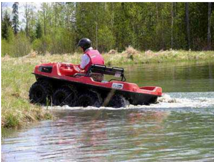
Figure A2-13 An Argo amphibious vehicle appropriate for survey in marshes. Note the problem of driving the Argo up steep banks out of waterways.
