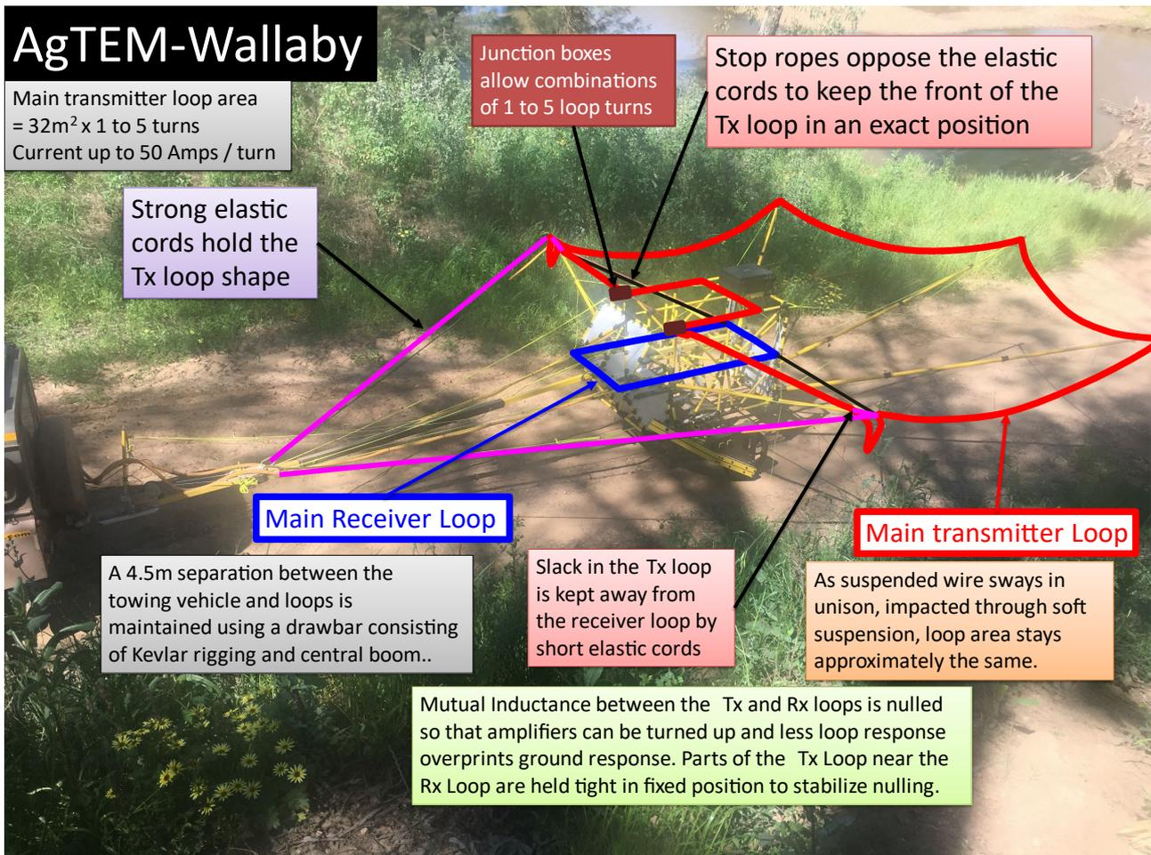
Figure 1. The key parts of the Wallaby towed transient electromagnetic antennae system. The Wallaby system is designed for efficient long-duration surveys across cleared agricultural land.
