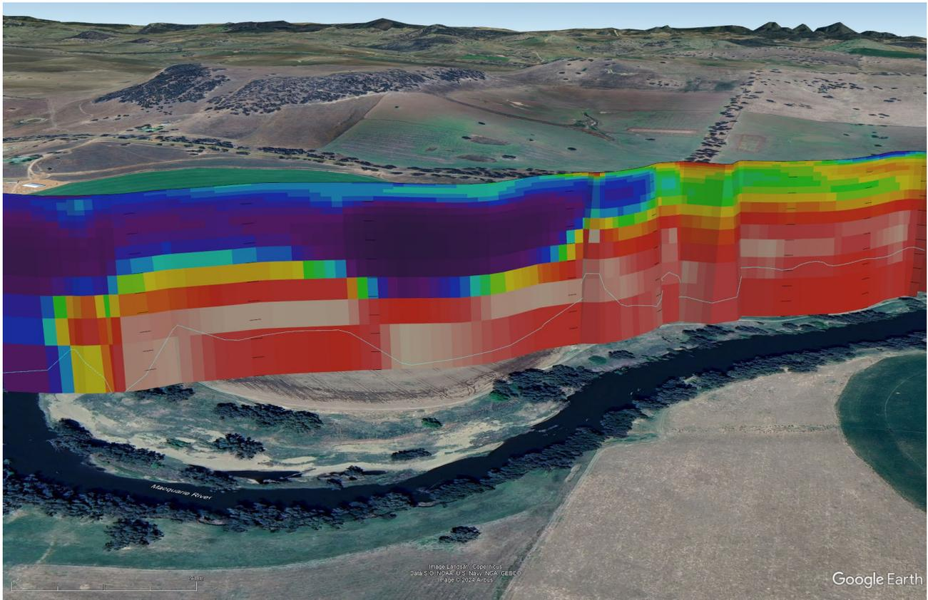
**Figure 10. Wallaby In-Loop transient electromagnetics. Modelled Resistivity projected up 160m (525 feet), 2 Parallel 1 Series Turns, 38Amps, 150 Watts.**
