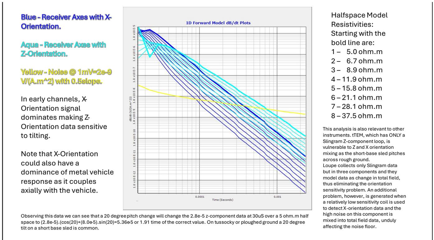
Figure 4. An example of type curves generated with TEMConfigurator. Wallaby front loop orientation comparison and signal stability.
