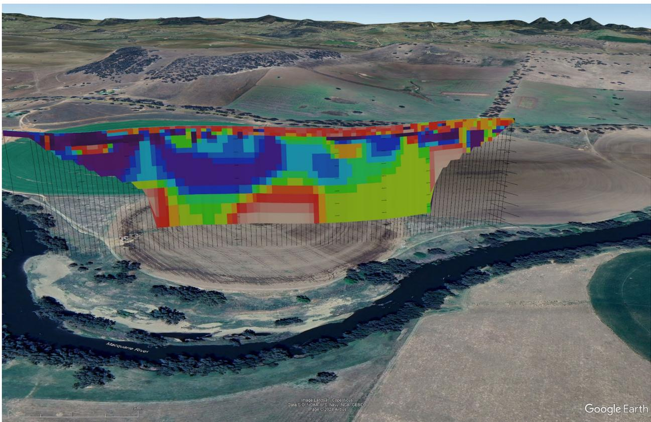
Figure 7. Direct Current Electrical Resistivity Tomography – Zhou array configuration. Modelled resistivity is projected up 160m using the colour distribution of figure 6.
