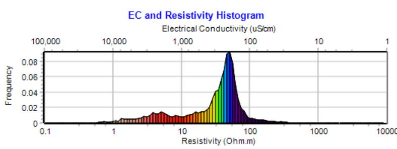
Figure 6. Wallaby transient electromagnetics resistivity distribution at the test site – used to colour the remaining figures.
