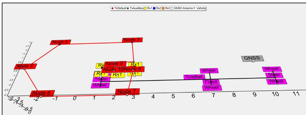
Figure 3. TEMConfigurator displaying loop coordinates from the Wallaby overlapping receiver loop configuration file.
