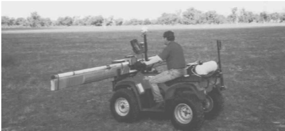
Figure 3.1 EM31 and DGPS set up for rice land classification. The boom is placed so as to straddle the quad bike. For production mode survey this placement is preferred by most Australian contractors, in preference to metal interference-free placement on a non-metallic trailer (from Shaw, 2001).
