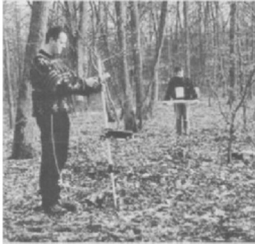
Figure 3.28 Iris Instruments Promis-10 wide coil spacing triple orientation receiver coil FDEM instrument
