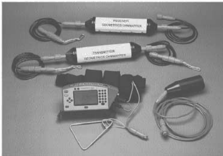
Figure 7.10 The OhmMapper with 2 transmitter and 2 receiver electrodes. A full system has 6 receiver electrodes (from www.geometrics.com ).
