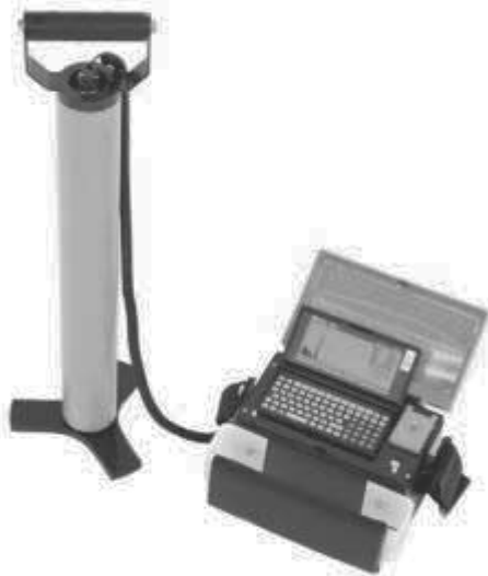
Figure 9.18 GF Instruments 512 scintillometer also available in a borehole version.
