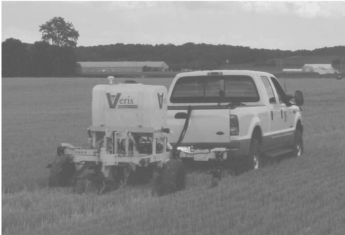
Figure 7.20 The Veris mobile sensor platform with electrodes sensing EC at 0.0-0.3m and 0.0 to 1.0m and pH at 0.1m depth every 12 seconds.
