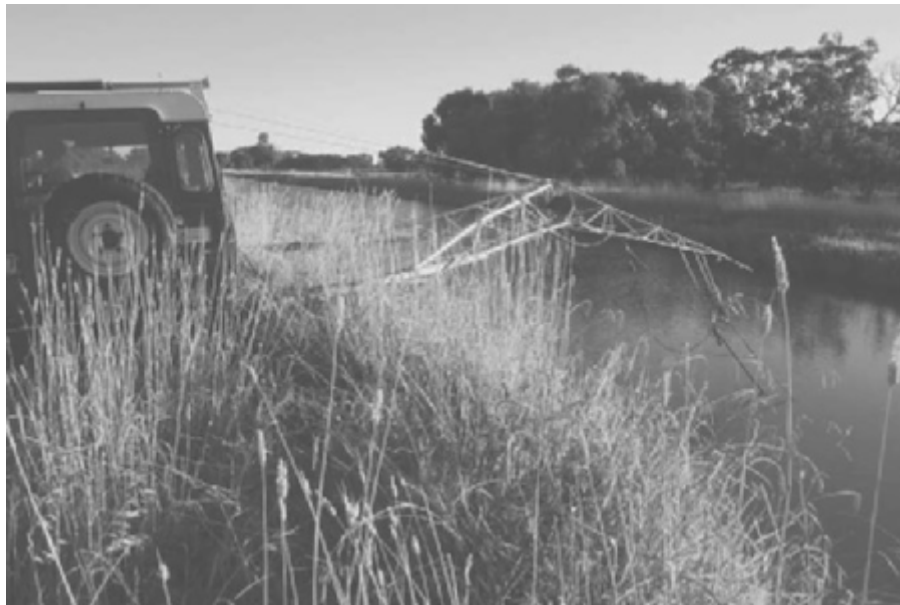
Figure 12.2 A foldable boom with a 6 metre reach, ability to straddle small trees and capable of towing geoelectric arrays using a spring attachment. The boom is raised/lowered using an electric winch on the roof.
