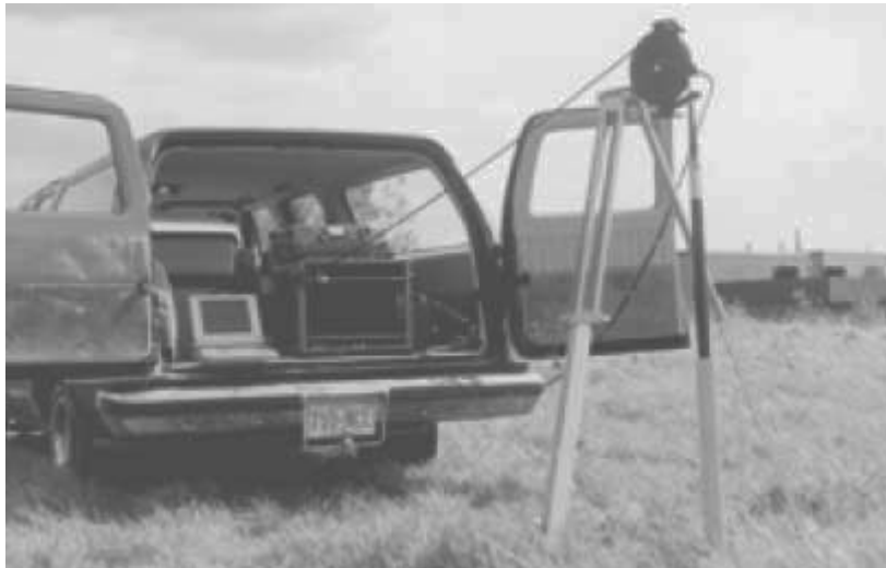
Figure 8.1 Geonics EM39 downhole electromagnetic induction logger.
