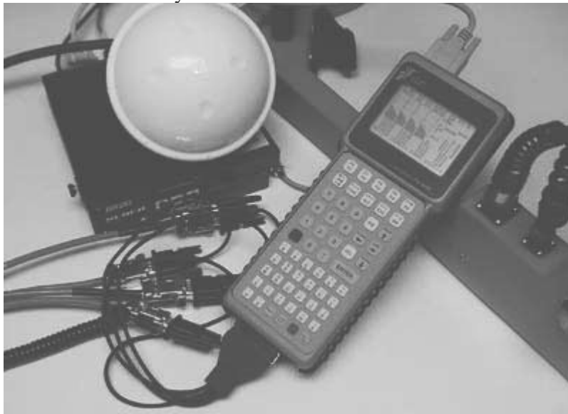
Figure 3.17 Allegro Pro4000 operating Geomar Multi31 (receiving GPS data and EM31 data from 3 different receiver coils).
