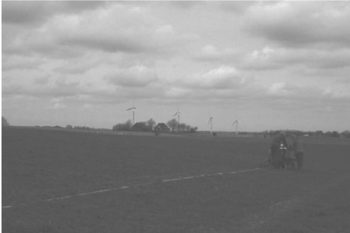
Figure 7.2 The PACES device being towed along near Aarhus, Denmark. The 300 kg 90 m long resistivity cable is being towed behind a tracked vehicle similar to the Australian ‘Dingo’ mini-earthmover. The system images to a depth of about 30 m provided that the ground is moist.
