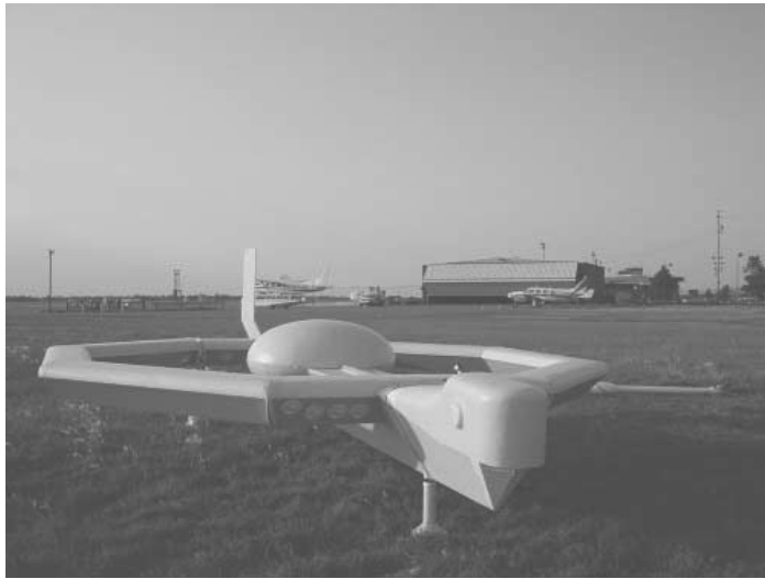
Figure 6.6 Aerotem helicopter-borne rigid transient electromagnetic system.
