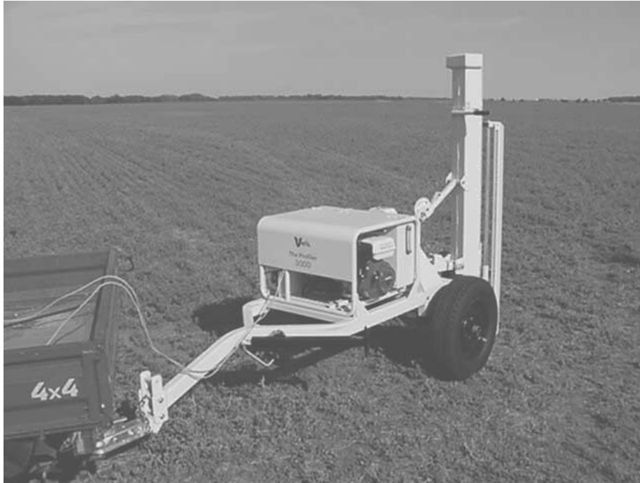
Figure 8.4 Veris Penetrometer with EC and pressure sensors.
