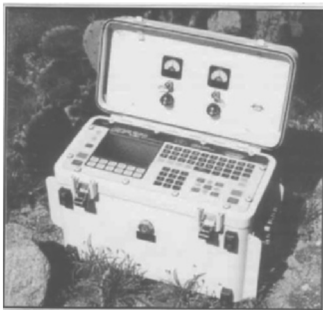
Figure 4.8 The Zonge GDP32-2 with an embedded NanoTEM Transmitter.
