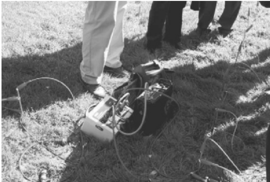
Figure 7.5 The ABEM SAS 4000 Terrameter and Lund Imaging System with electrodes laid out in a miniature array for demonstration purposes.
