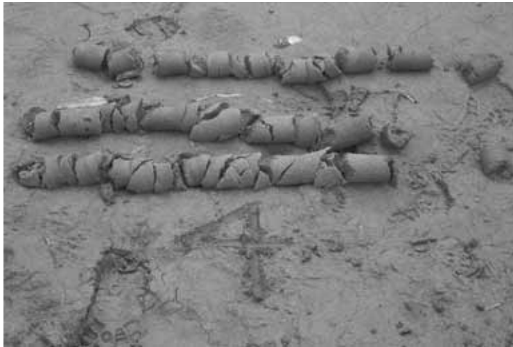
Figure 12.8 Coarse Sand of a prior stream evident under the kink in the canal presented in Figure 12.5. Three x 700 mm samples with 100 mm of silt impregnation at the tops (Right) are displayed.
