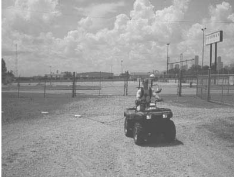
Figure 7.11 A capacitively coupled resistivity meter towed behind an all-terrain vehicle in Nebraska. The capacitively coupled resistivity meter (the cable and white tubes) consists of a coaxial-cable array with transmitter and receiver sections. (Source – USGS OGW Branch of Geophysics website)
