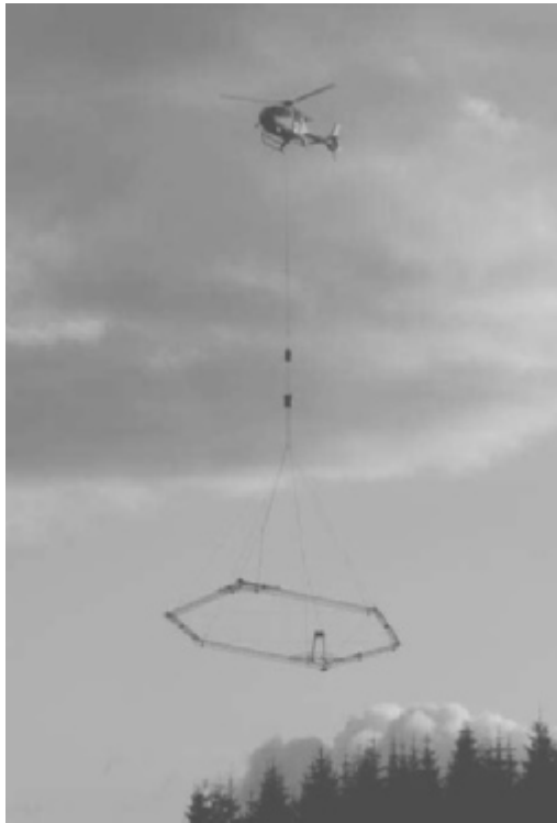
Figure 6.2 SkyTEM rigid helicopter-borne transient electromagnetic system with null coupled receiver coil.
