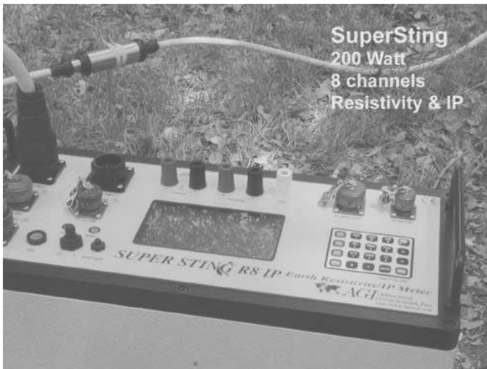
Figure 7.8 The AGI Super Sting R8 IP Earth Resistivity/IP Meter.
