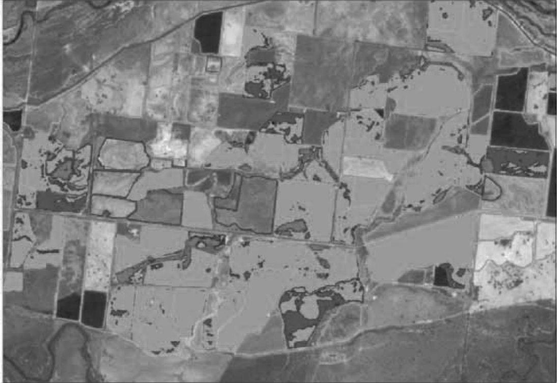
Figure 3.3 Rice land classification derived from EM31 surveying assisted by drilling and soil sampling. Red - Unsuitable, Blue - Suitable for crop rotation, Green – suitable (from Shaw 2001).
