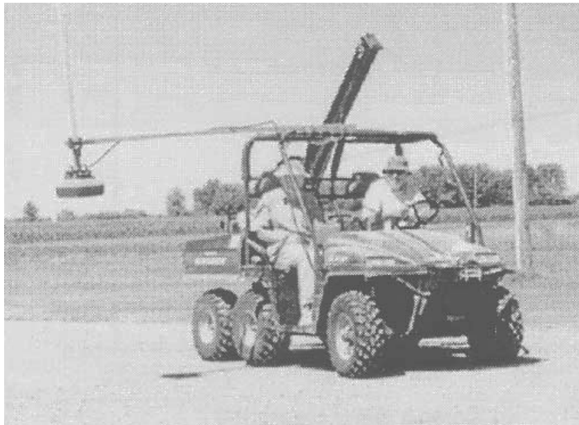
Figure 9.20 An elevated 500-MHz ground penetrating radar (GPR) system being used to measure soil moisture content using surface reflection amplitude (from Huissman et al., 2003).
