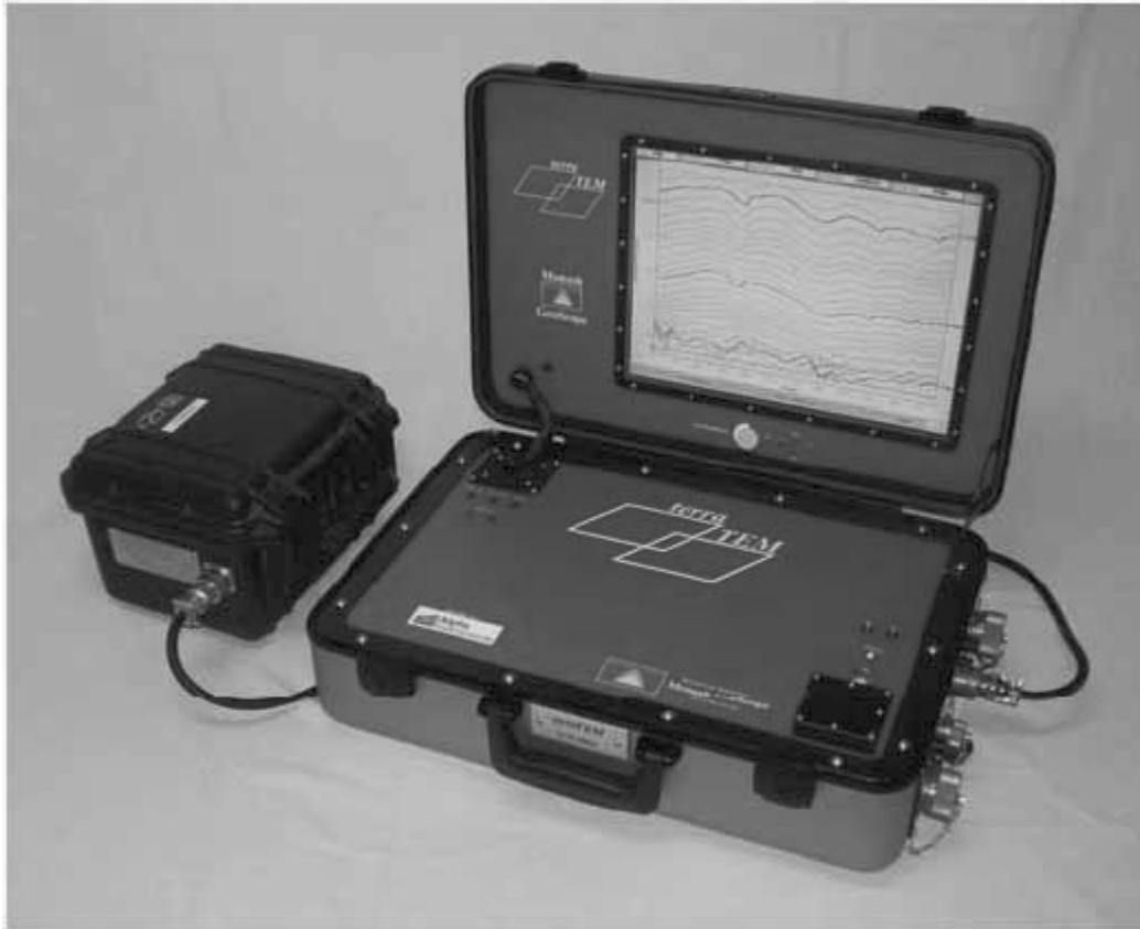
Figure 4.5 The TerraTEM system incorporating a TEM transmitter, receiver and controller with a colour touchscreen (battery on left).
