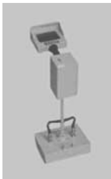
Figure 9.9 The COS Senci-On \beta 2 ground penetrating radar instrument claimed to be able to indicate water leakage from pipes.
