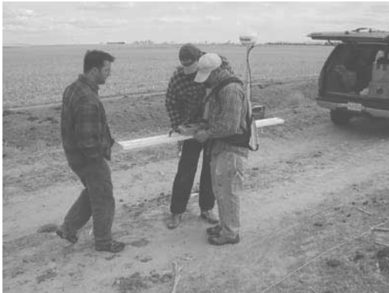
Figure 3.22 Eric White (USGS, OGW, Branch of Geophysics), conducting a geophysical survey in Nebraska using a Geophex GEM 2 multi-frequency electromagnetic sensor.
