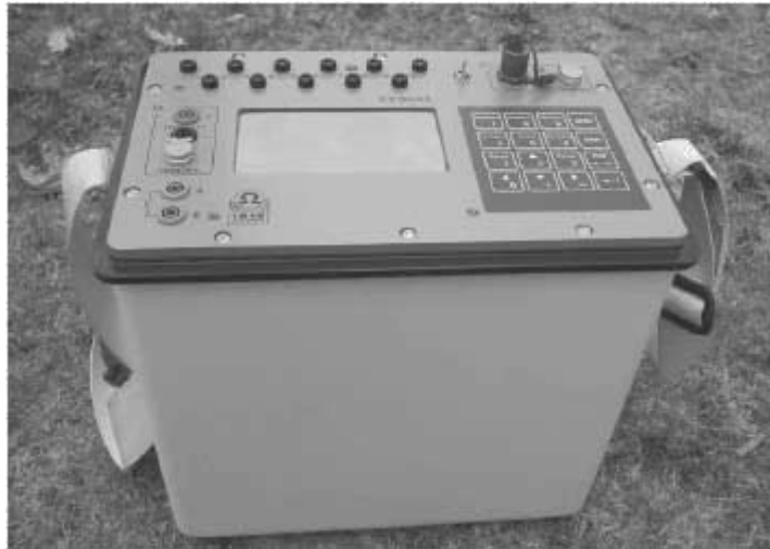
Figure 7.15 The Iris Instruments Syscal Pro resistivity imaging device.
