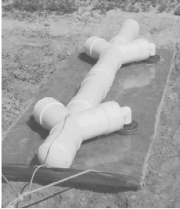
Figure 3.14 DUALEM 2 on a highly robust sled with lots of impact absorption for reducing movement related noise. (Photo: A. Schumann, University of Florida)
