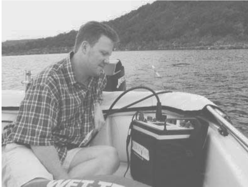
Figure 7.9 The AGI Marine Resistivity Imaging System
