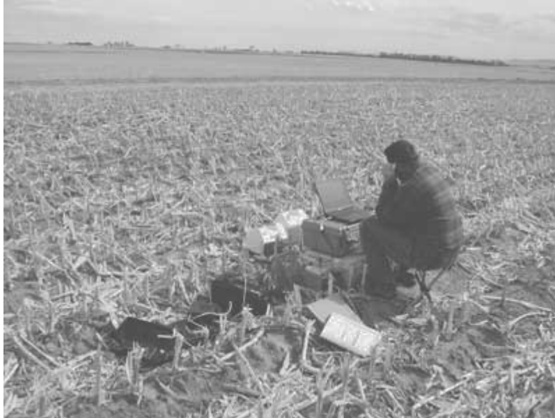
Figure 9.19 Conduct of a seismic survey in Nebraska (from USGS, OGW, Branch of Geophysics web site).
