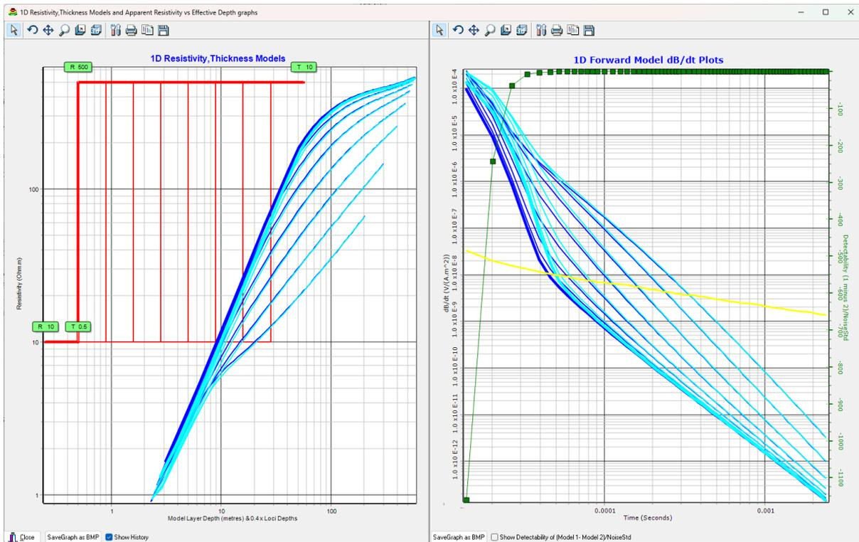
Notice the change in early times. Getting filters wrong will result in inversions generating artefacts near the surface, and, if inversion cannot accommodate the error this way, it will typically either drop the layers modelled deeper into the earth or generate a spurious conductive layer that absorbs deep response and hides deep features.
