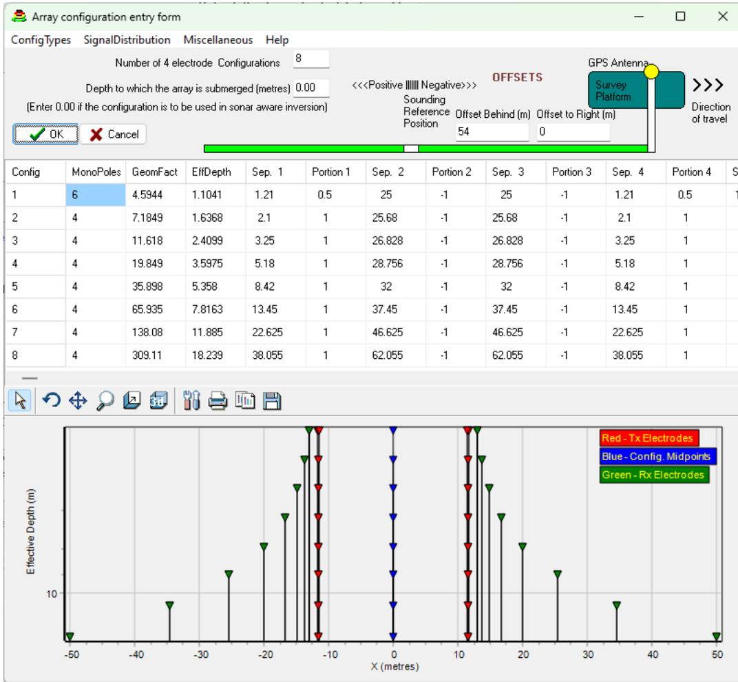
Note that this facility breaks long electrodes up into parts when they are close to other electrodes so there are, in this case, 6 monopoles in quadrupole 1.
