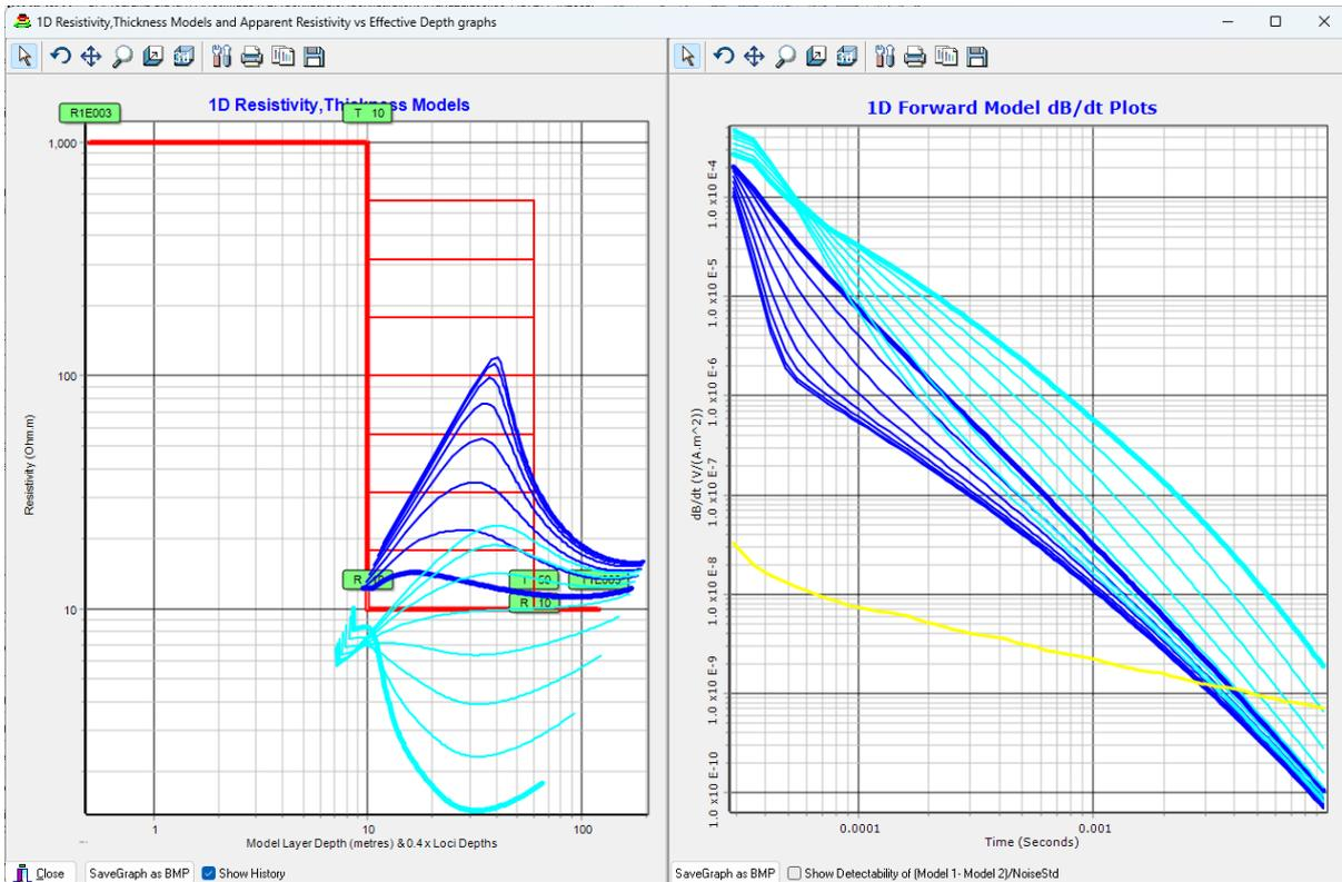
Notice how the type curves for the previous models are still shown on graphs. This is handy for comparison, including tweaking of configuration parameters – that is it is not only layered model parameters that can be changed between runs such as has been done in this example. Try toggling the ‘Show History’ and ‘Show Detectability’ check boxes to change what is displayed on the graph. Above the detectability graph has been turned off to reduce complication.
