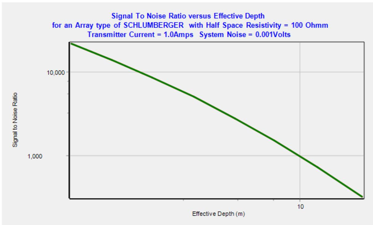
Under 'Miscellaneous' there are options for changing parameters used to determine this graph. Should you go and change configuration parameters then you can replot and the remaining plot will remain superimposed for comparison. As an exercise, if you change to a bipole-bipole configuration with  $a=5$  metres and  $n=8$  then redisplay then you will see the merit of the Schlumberger array. The bipole-bipole array is displayed in red below – see that it lacks both depth range and signal strength:
