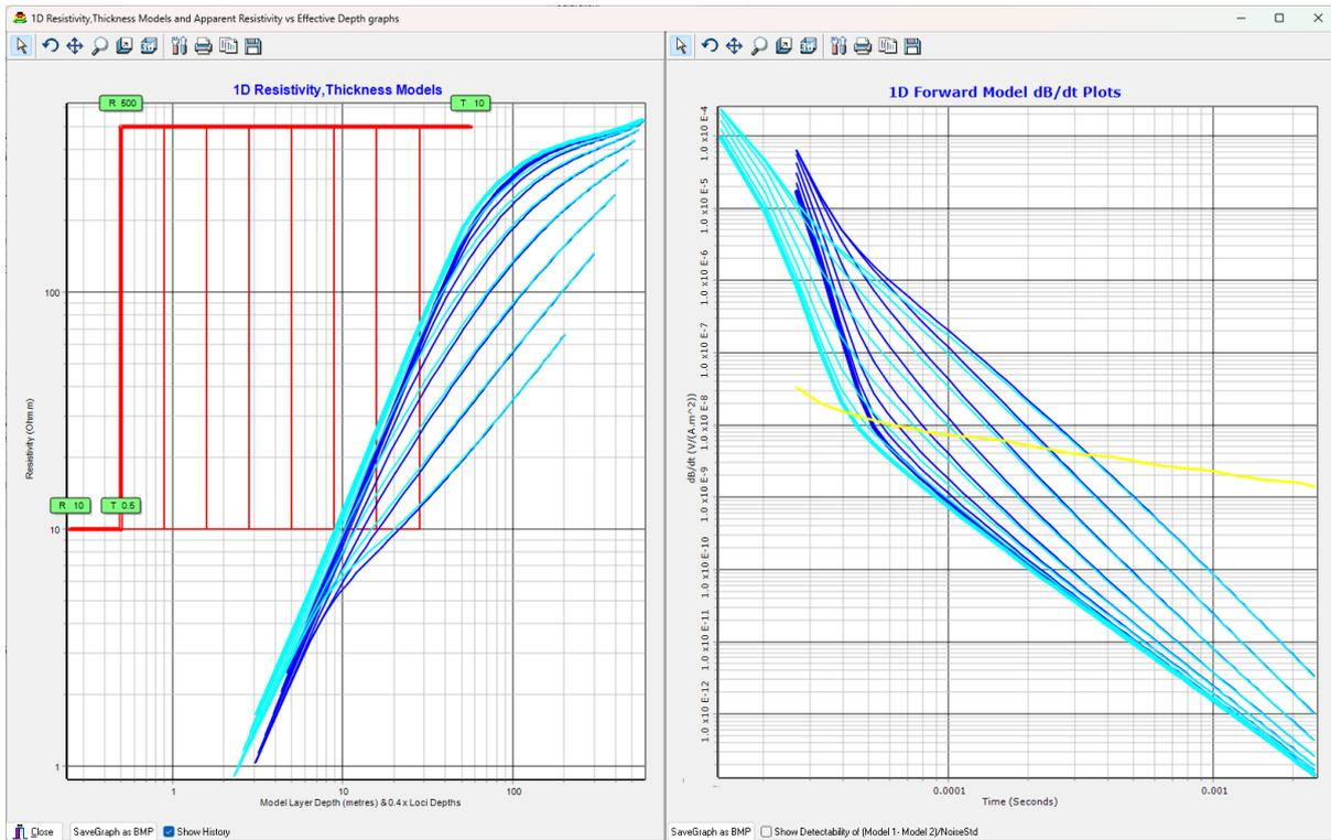
Notice that the extra 10uS makes it hard to resolve the contrast in the 10 ohm.m layer until it exceeds 1 metre in thickness. Also notice that changing filters and changing ramp time have similar effects on forward models if the early channels are excluded from observation.
