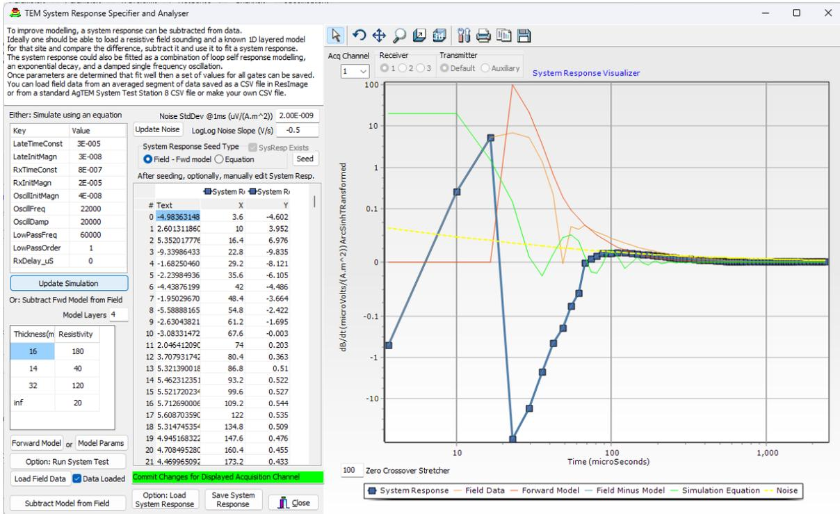
Figure 12 The system response display of TEM Configurator.
