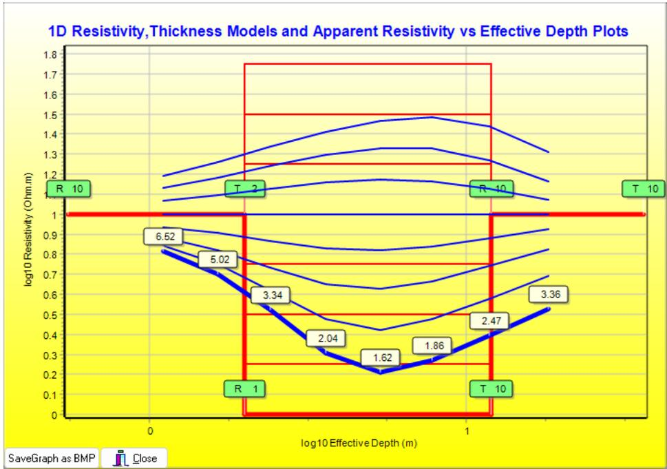
This set reveals contrasts observed in apparent resistivity data for models of the type from top to bottom of conductive-resistive-conductive and resistive-conductive-resistive as the middle layer ranges from 1 ohm.m through decade steps 1.8 ohm.m, 3.1 ohm.m, 5.6 ohm.m, 10 ohm.m, 18 ohm.m, 31 ohm.m and 56 ohm.m. Because there is considerable contrast between adjacent type curves we can have confidence that this array will resolve these types of models well.
