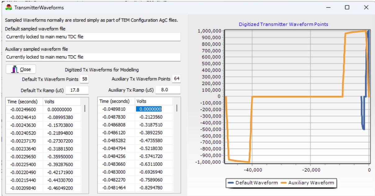
Figure 11 Transmitter Waveform display of TEM Configurator
