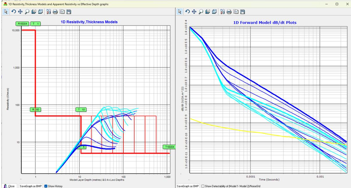
Resistive layer thicknesses are 10, 18, 31, 56, 100, 180, 310 & 560 metres. See that the main difference is a drop in effective returned signal strength, particularly at earlier times. This means that if Wallaby, with one Tx loop turn and 32 Amps, is airborne it can only distinguish basement in this set of models to a depth of <100m but if on the ground it can distinguish basement to a depth of <180m.
