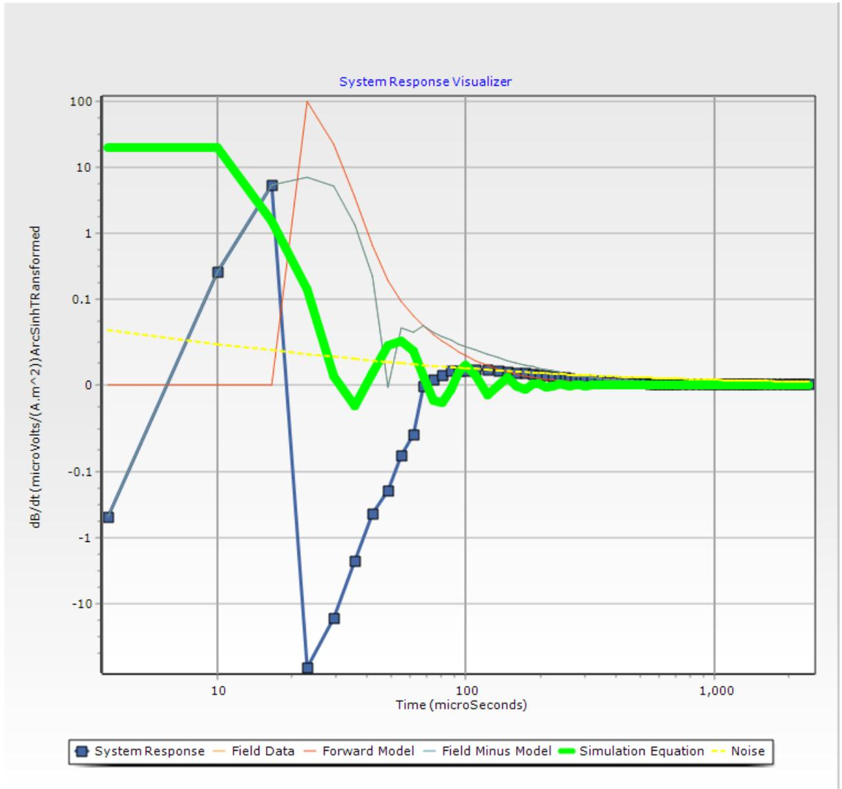
This equation response is not active in this configuration so its effect is nil unless used to seed the system response. If the forward modelling option is used, parameters such as delays on other forms will affect the model, shown in red, here. If you iteratively change the equation variables, you will find you can very closely mimic the system response.
