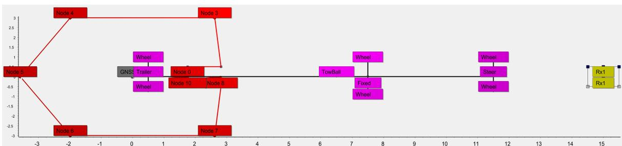
Figure 5 Plan view of AgTEM-Wallaby slingram-only configuration
