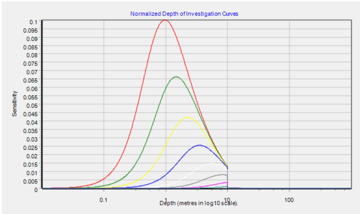
See how signal contribution basically disappears once the conductive basement is reached. This is why direct current resistivity methods are recommended more for use detecting resistive features, while electromagnetic methods are used for detecting conductive features.
