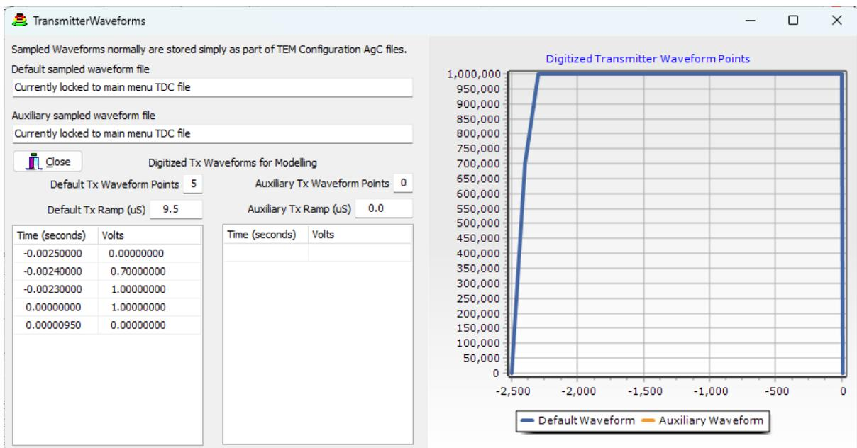
The ramp is a read only parameter here, driven by the last line of the waveform description table. Modelling software AarhusInv64.exe operates only with the entire waveform and treats the ramp only as a 'sub-wavelet'.
