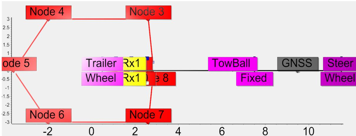
In this configuration, transmitter and receiver loops overlap so that mutual inductance is stably nulled. The actual receiver position is replaced by a dipole centred receiver as this is how it is modelled in inversion software. The actual shape and position is slightly different. Similar modelling simplifications are applied to many airborne systems in examples provided. The graphical display is suited to quickly making configuration description mistakes obvious.
