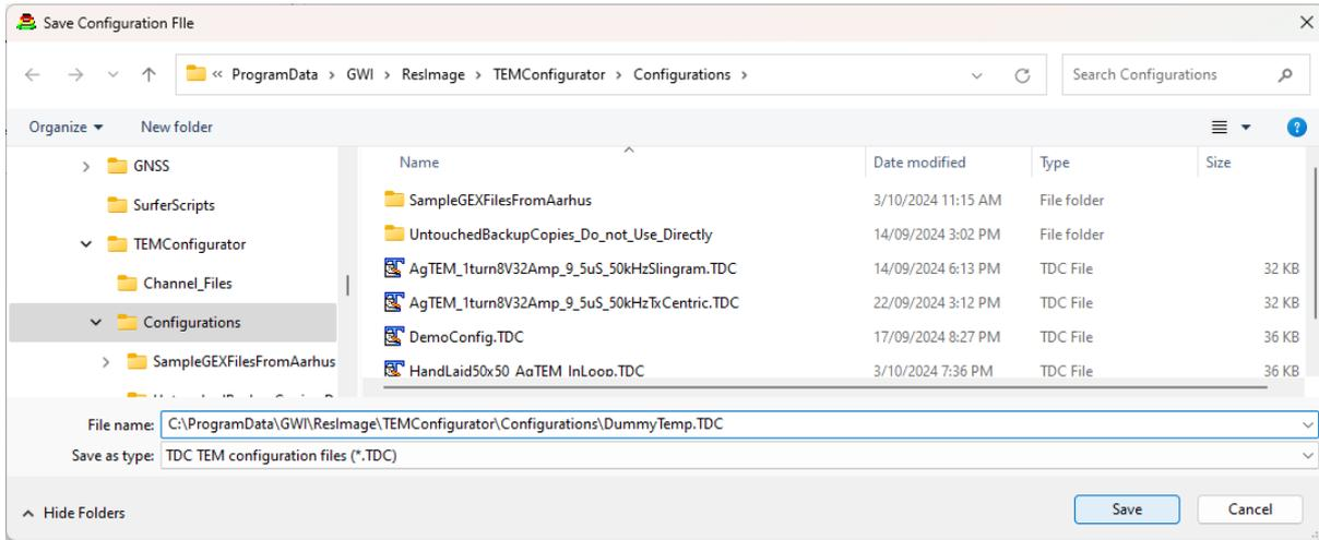
Saving back to the original file name would be detrimental as we just wiped out the filters so it is safer to save to an obviously temporary filename. The forward modeller reads from the file so any changes not saved will not have an effect.
