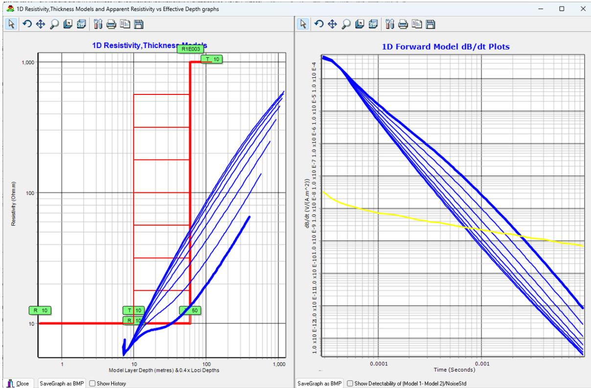
Now we see that type curves for the more resistive middle layers are very close together indicating a very poor resolution of this type of model contrast.
