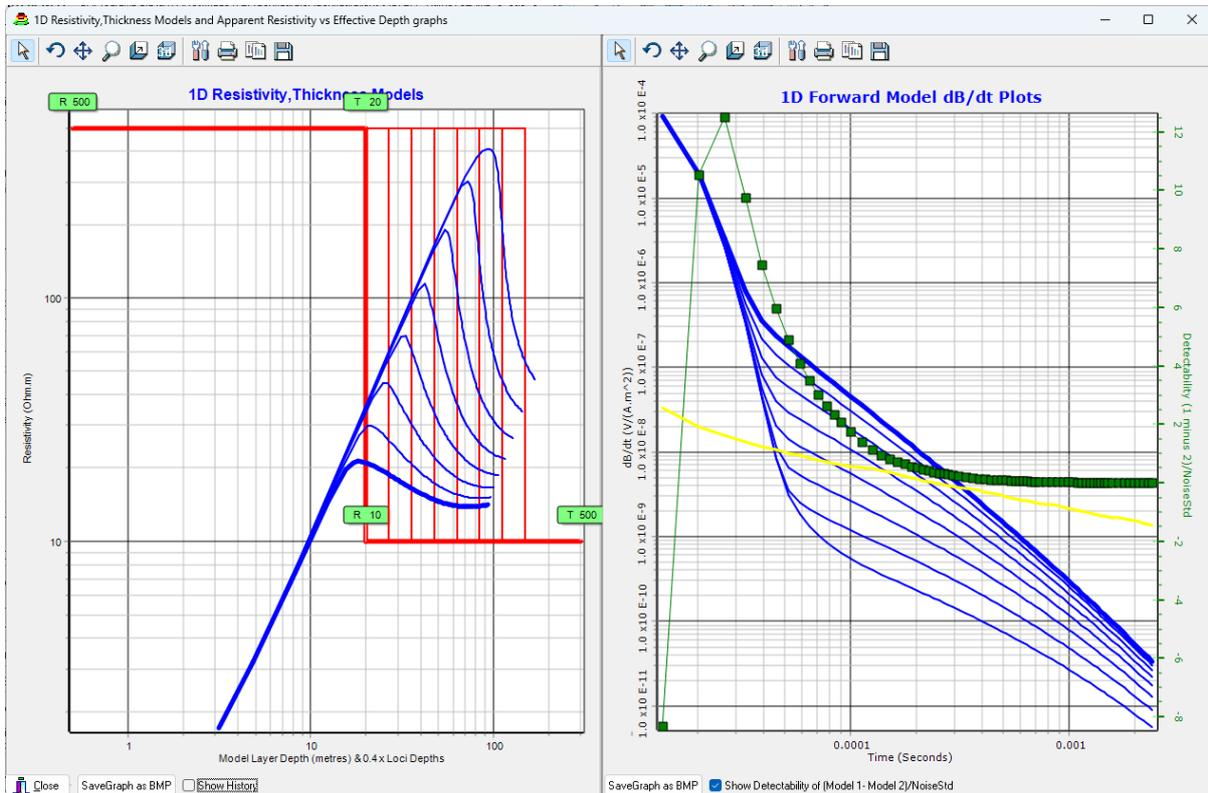
The results show excellent contrast between type curves however the distinguishable segments of the curves for models with depth to basement exceeding 60 metres drop beneath the designated noise level of  $2e-9$   $V/(A.m^2)$ . This noise level is chosen assuming rough travel over tussocky vegetation and with systematic noise sources poorly resolved as can be normal under production pressure. If deeper basement were to be resolved,
