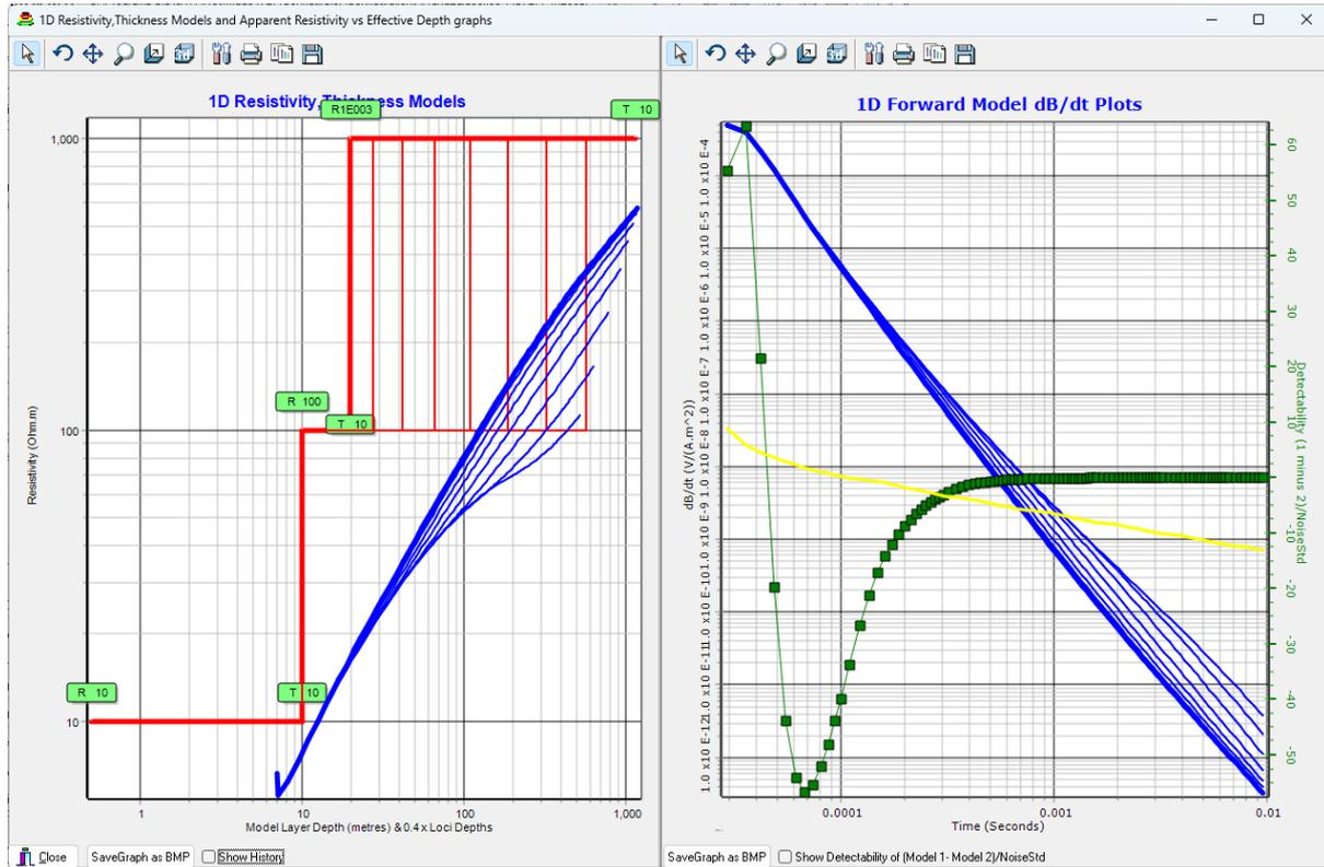
See that the resolution problem remains whether we adjust resistivity or thickness of this middle layer. It is a problem of equivalence. Despite resistivity methods obtaining more signal from resistive features, while electromagnetic methods obtain less signal from resistive features, if considered in terms of signal returned for unit of power delivered, they both lose most resolution for cases where conductive layers overly resistive layers.
