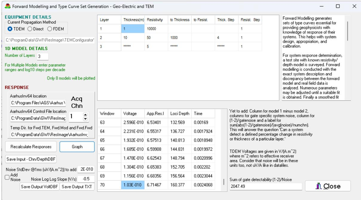
Figure 14 The forward modelling form of TEM Configurator.
