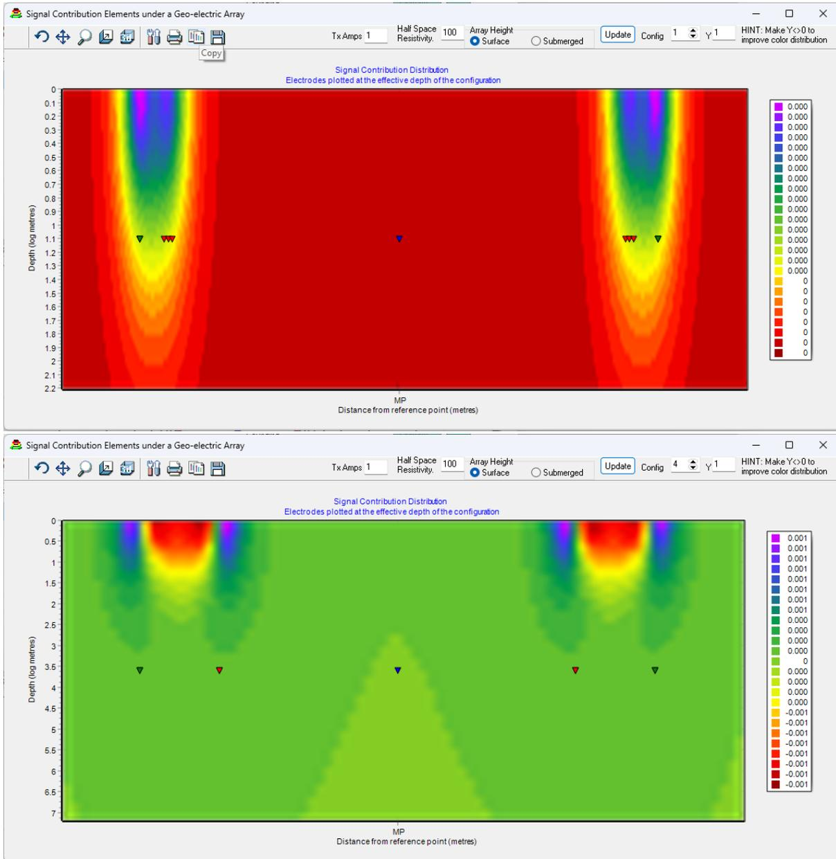
Results for both quadrupole 1 and quadrupole 4 are displayed. Notice how the contribution distribution becomes complicated as electrode separation is increased. It is far from the 1D layered case suggested by the NDIC curves plotted previously so remember that electric, and electromagnetic, methods are strongly dependent on 3D distributions of conductivity.
