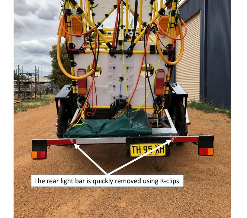
The rear light bar wiring is connected here so it can easily be fully removed
