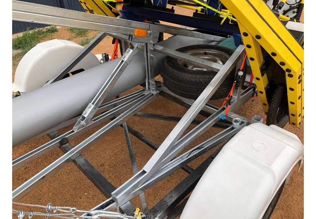
AgTEM-cart is secured at the tow hitch and each side of the undercarriage cross-member. On the cross-member there are polyethylene guide blocks designed to precisely guide AgTEM up the float trailer skids. The distance between the skids is thus critical. The angle and height of the skids also is critical to the guide blocks sitting level. Straps tie down each side of the cross-member.
